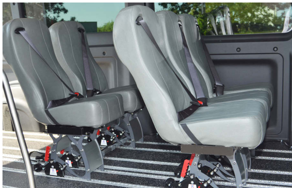
Our exclusive SmartFloor system can provide unlimited seating and wheelchair layout options.
